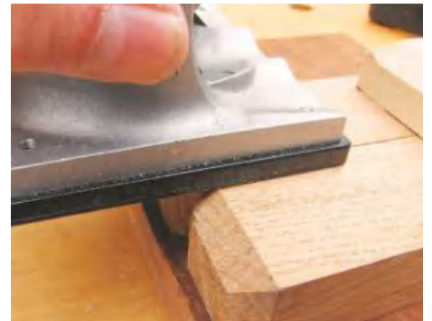
STEP 9. Plane the two end pieces to size, and then cut slots. Next, rout a chamfer around their lower edges
